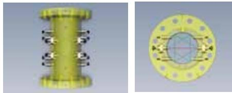
The Q.Sonicmax uses three pairs of direct cross X paths in the same plane and two swirl double reflection paths culminating in a sophisticated acoustic imaging and interrogation of the gas stream.
