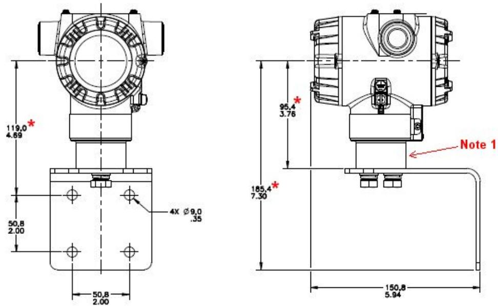
Figure 3 – STT850 with adapter housing - Horizontal Wall Mounting
