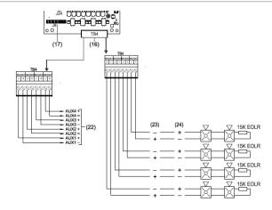
Marking indicates output signal polarity when the circuit is active. Polarity reverses when the circuit is not active. Wire notification appliances accordingly. Notification appliance polarity shown in active state.
