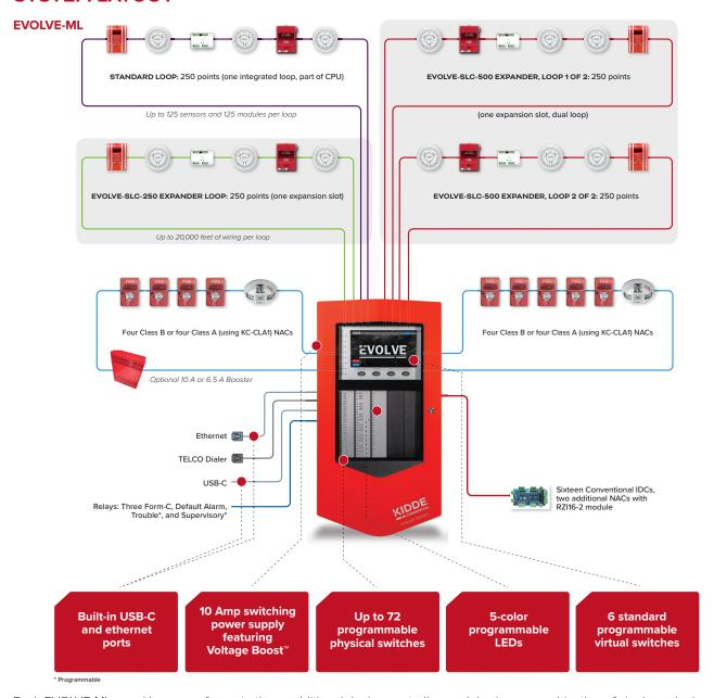
Each EVOLVE-ML panel has room for up to three additional device controller modules in any combination of single or dual device loops. EVOLVE-ML comes with one built-in loop that supports up to 125 detector and 125 module addresses.
