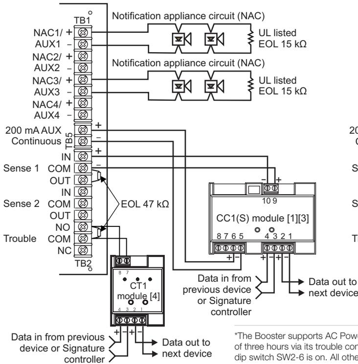
\*The Booster supports AC Power fail delay of three hours via its trouble contact when dip switch SW2-6 is on. All other troubles are reported to supervising module or panel without delay via Sense inputs.
